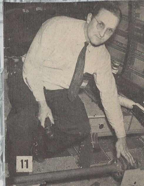
11. WILLIAM BLISS, M554, suggested torque tube assembly No. 5103783 be completely assembled in one department, aligning six pulley brackets. Cuts down reworks, saves time.
